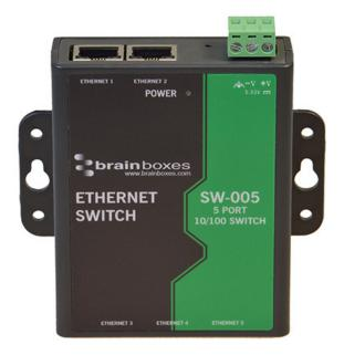
Switches control the flow of network traffic based on the address information in each packet. A switch learns which devices are connected to its ports (by monitoring the packets it receives), and then forwards on packets to the appropriate port only. This allows simultaneous communication across the switch, improving bandwidth.
